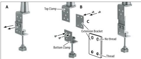
\*VERY IMPORTANT: Install screws through the INSIDE of the top clamp, and through the OUTSIDE of the bottom clamp in order to keep clamp intact and prevent damage.
