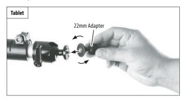
Insert the ball into the back of the tablet holder and tighten the ring to secure.
