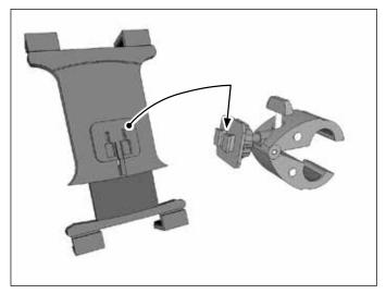
Unscrew mount's knob to loosen grip. Place the mount around pole as desired, then retighten knob to secure.
