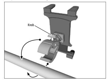
3 Insert device by pushing down on the lower legs of the spring-loaded holder.
