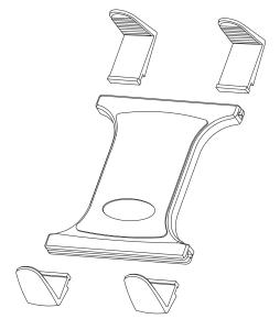
Assembling the shaft arm to the tablet holder and magnetic mounting plate
