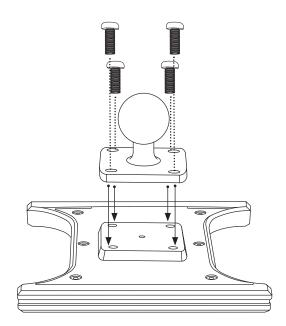
Installing the adjustment legs to the tablet holder
