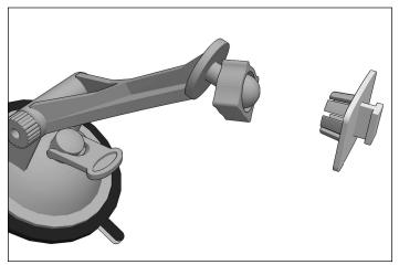
Insert Single T-Tab into slot on satellite radio cradle (sold separately, not included).
