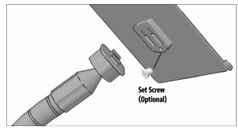
Optional: Attach included metal conduit to console to minimize vibration.
