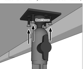
Adjust mount to desired position via the adjustment knobs.
