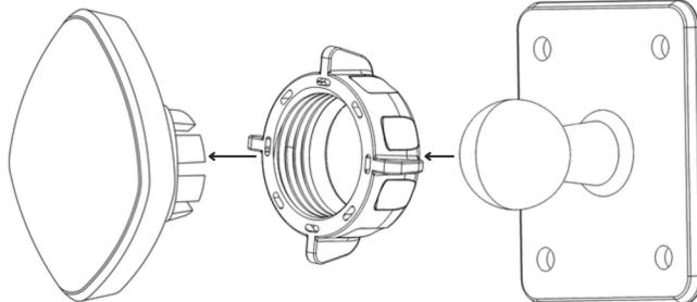
**4 Installing the Magnetic Plate on Your Device**
