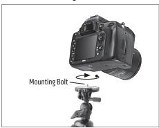
2 Loosen the adjustment knob to change position and retighten to set.
