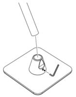
Attaching the Adapter to the Pole
