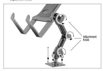
4 Mount printer by pushing down on bottom spring-loaded legs; adjust holder and support legs as needed.
