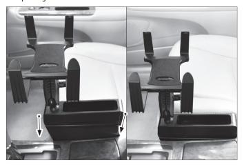
2 Attach the adapter to the holder with the provided screws. Combine the Robust Shaft to adapter and seat mount and tighten adjustment knob to secure.
