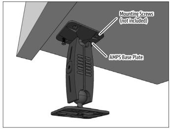
**3** To adjust pedestal position, loosen the hex bolt with Allen wrench and reposition. Retighten to set.
