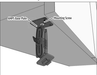
2 Loosen adjustment knob to adjust angle of pedestal and position of Dual-T adapter plate. Retighten to secure.
