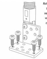
Rotate or reposition the bracket as needed to fit your vehicle's floor or console layout.
