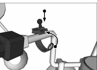
Using two hands, insert the phone into the holder by pushing the device into one of the spring-loaded legs. Expand the other leg and fully insert device until it lays flat against the
