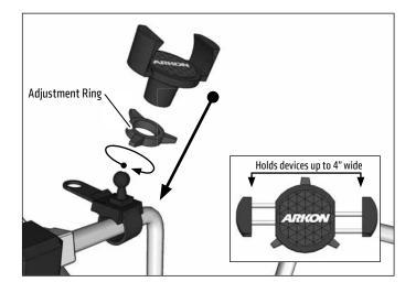
4 Remove mount by pulling up release tab and pushing strap back through slot.
