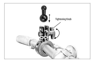
Unscrew tightening ring from RoadVise holder. Place adjustment ring over 17mm ball end of mount then snap the RoadVise Universal Smartphone holder onto 17mm ball and tighten ring. Set to desired position.
