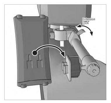
**13** To mount a device, push down on legs and place in holder.
