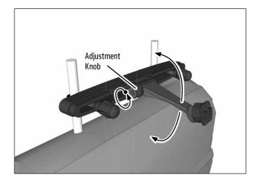
4 Insert iPad mini or midsize tablet by placing it on the 2 lower legs and pushing down on the spring-loaded bottom of the holder. Loosen tightening ring to adjust position and angle. Retighten to set.
