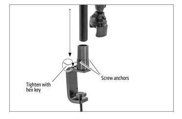
2 Loosen the screw anchor at the base of the stand and remove the extendable pole from the stand.
