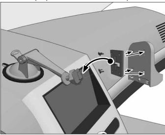
For satellite radio cradles (sold separately, not included) without 4-Hole AMPS pattern, insert Single-T slot to pedestal head.
