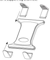
Optional - Installing the leg stoppers Locate the packaging containing the 4 leg stoppers. Insert the leg stoppers into the holder's leg channels.
