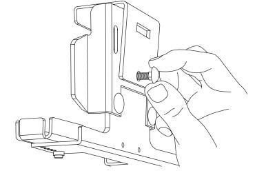
Pull screw out from the back of the locking arm
