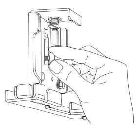
Re-insert screw to the front of the holder going through the
