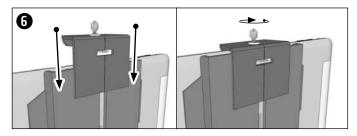
To lock down tablet, close down on the locking arm on the top of the tablet and lock with key (included).
