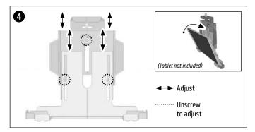
Unscrew the three screws/washers at the back/center of the holder to adjust the tablet holder's height to the tablet (not included). Retighten the screws/washers to secure.
