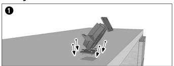
Using a screwdriver and/or drill, attach the metal AMPS mounting base to a flat surface with 4 screws (not included).
