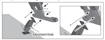
Unscrew the three screws/washers at the back/center of the holder to adjust the tablet holder's height to the tablet (not included). Retighten the screws/washers to secure.
