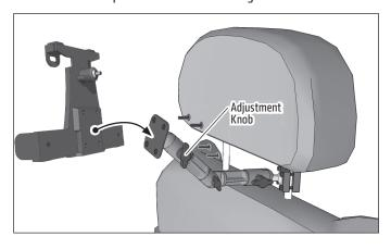
2 Loosen the adjustment knob on the pedestal, remove the Dual T-Tab adapter, and position the pedestal over the mount's ball. Retighten knob and set pedestal to desired angle.
