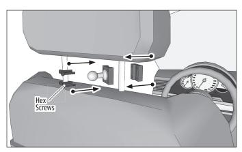
3 Attach the holder to the mount by adding the screws through AMPS adapter to the back of the mount. Loosen adjustment knob to set desired position of holder and retighten.
