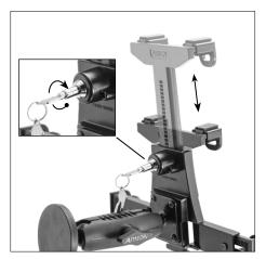
Insert tablet into holder. Adjust top of holder to fit tablet. Push button in on back lock to secure tablet.
