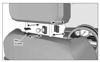
3 Attach the holder to the mount by inserting the Dual T-Tabs into the holder's Dual T-Slots and pushing down to lock. Loosen adjustment knob to set desired position of holder and retighten.
