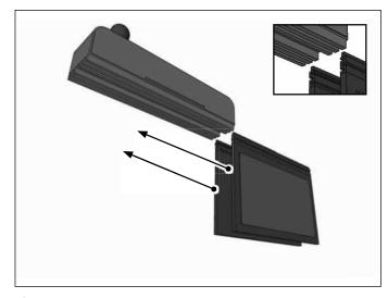
Attach adapter to the pedestal's rubber ball, then attach tablet holder to the adapter by sliding the adapter's Dual T-Tabs into the holder's Dual T-Slots.
